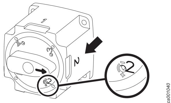
Remember your torque settings by placing your own markings on the four areas on the housing.
