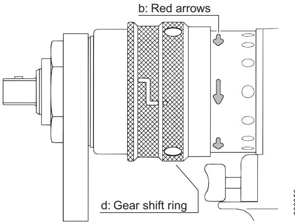
The red arrows indicate the direction of running. I.e. the machine will run counter-clockwise when started.
